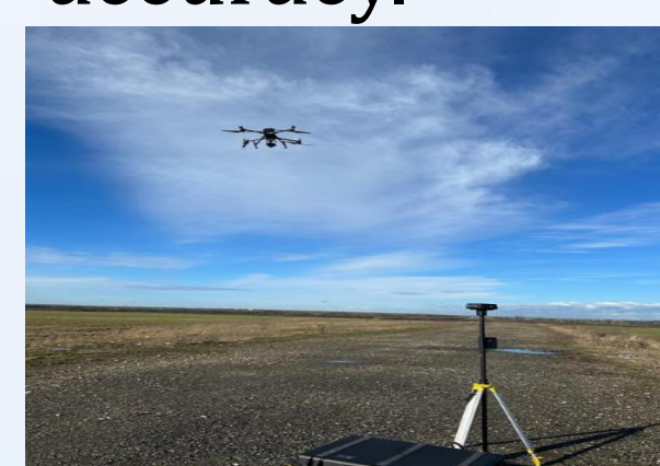
Figure 2. DJI 300 RTK matrix with D-RTK 2 GNSS mobile station
