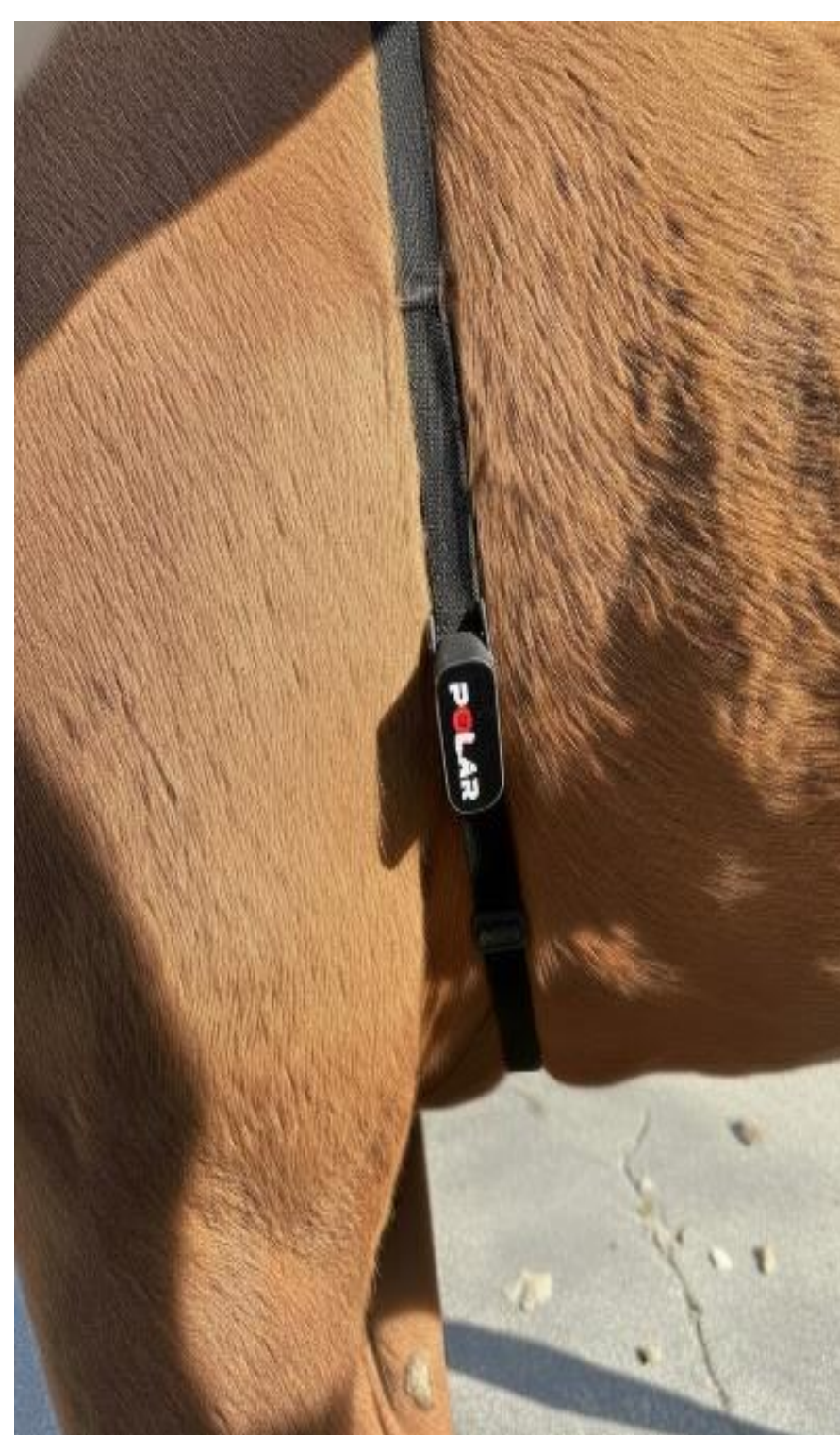
Figure 1: Placement of the Polar Equine H10 heart rate sensor on the horse's thoracic region.
